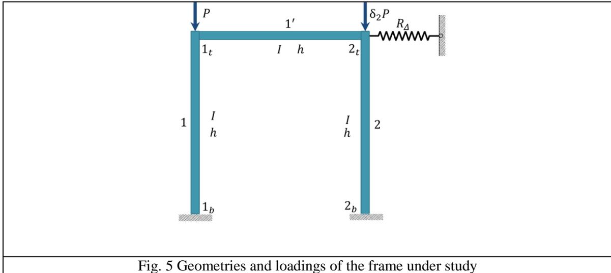
Fig. 5 Geometries and loadings of the frame under study
