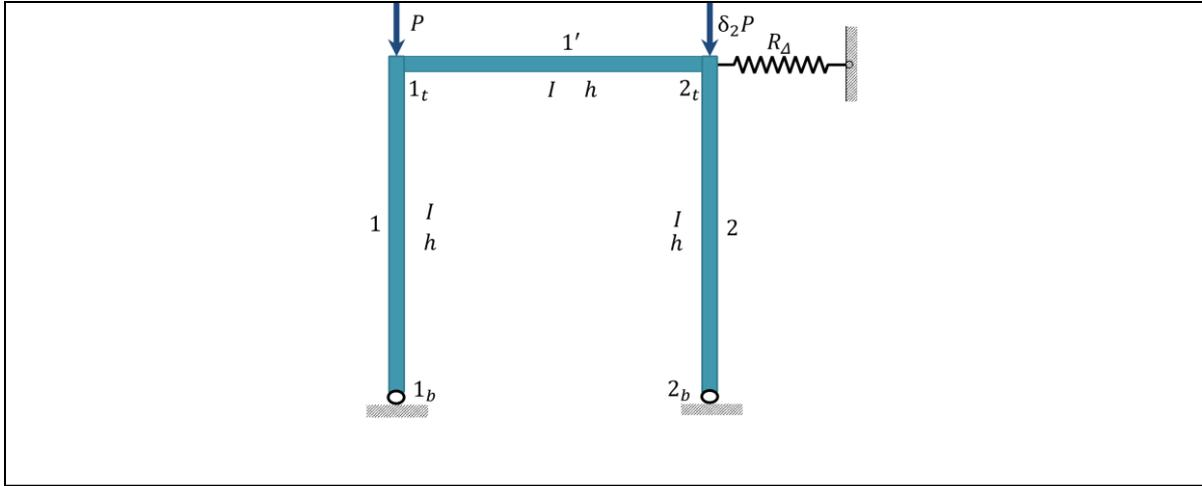
Fig. 3 Geometries and loadings of the frame under study
