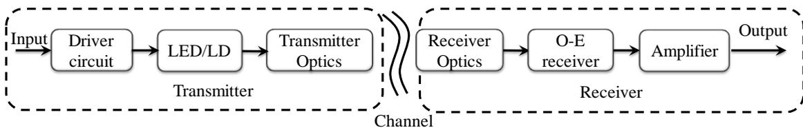
Figure 1: A block diagram of a VLC system.
