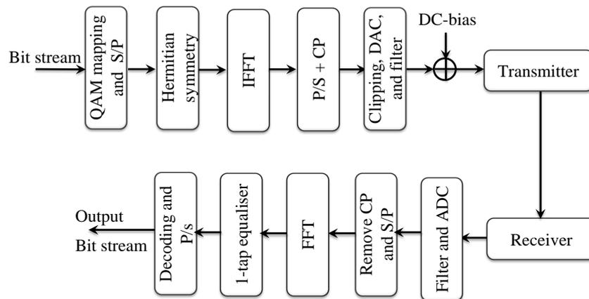
Figure 13: A schematic block diagram of the DCO-OFDM signal generation and demodulation.
