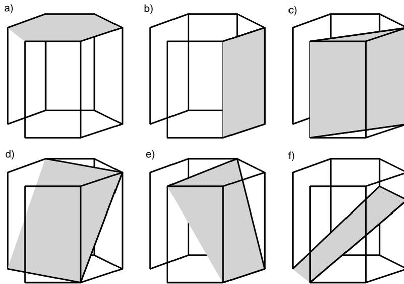
Figure 5: Important growth orientations in hexagonal GaN: a)  $c$ -plane (polar), b)  $m$ -plane (non-polar), c)  $a$ -plane (non-polar); d)-f) examples of semi-polar planes, d)  $11\bar{2}2$ , e)  $10\bar{1}1$ , f)  $10\bar{1}3$ . The plane shaded in grey represents the GaN crystal plane parallel to the substrate surface. It is shown in relation to a hexagonal prism larger than the conventional unit cell of GaN, and the crystallographic  $c$ -axis is vertical in each case.
