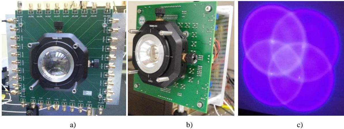
Figure 19: A MIMO VLC demonstrator developed for the UP-VLC project, showing a) the transmitter system, b) the receiver system [33] and c) an image of the 4  $\mu$ LED beams as seen at the receiver plane.
