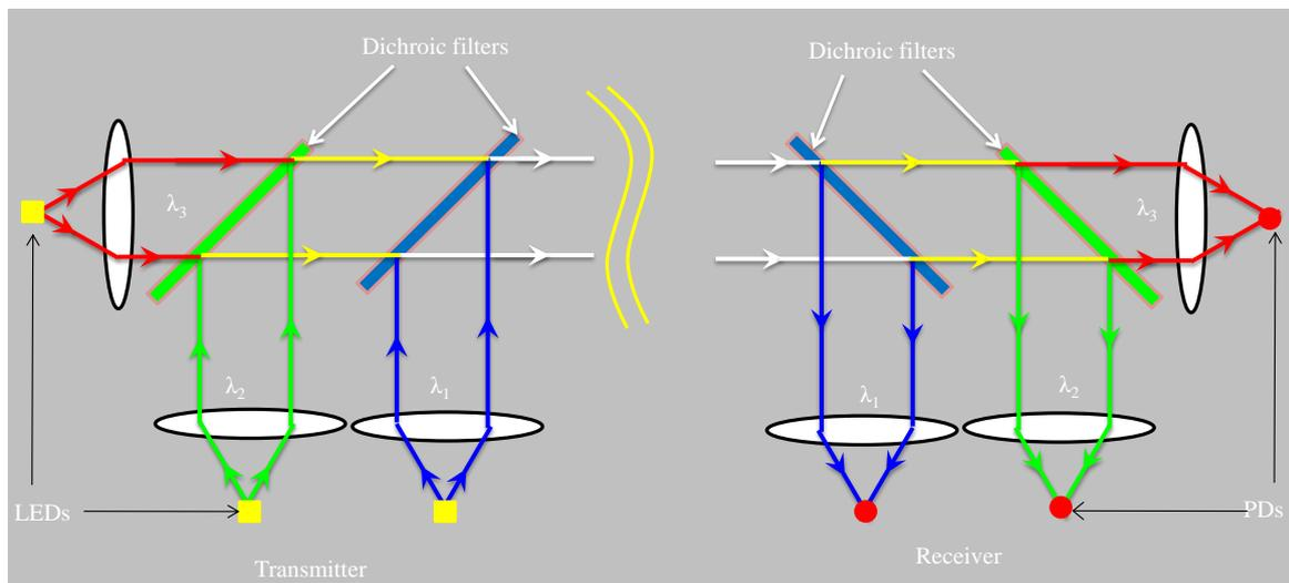
Figure 20: Schematic of a WDM-based VLC system.
