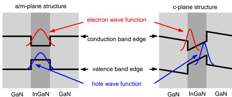
Figure 6: Illustration of the QCSE, where the vertical axis represents potential energy and the horizontal axis distance in the growth direction (the typical QW thickness is 2-3 nm). In  $c$ -plane GaN LEDs, the net electric field leads to a separation of the electron and hole wavefunctions and thus reduced carrier recombination rates.
