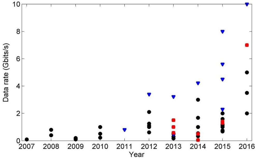
Figure 10: Progress in the reported data rates using visible GaN LEDs, black (circular) dots representing demonstration without any multiplexing, red (square) those with spatial multiplexing and blue (triangular) those with WDM.
