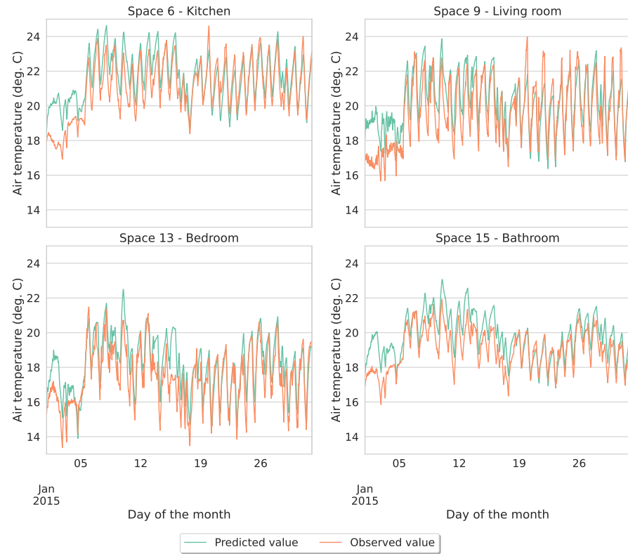
Figure 5.7: The observed and predicted values for the air temperature in four rooms of house 0 throughout January 2015. The rooms depicted in the top row are the kitchen (space 6) and living room (space 9), and in the bottom row is the bedroom (space 13) and bathroom (space 15).
