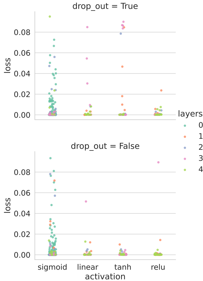
Figure 4.7: Overview of hyperparameter search showing the loss (mean squared error (MSE)) for with and without dropout and separated for each hidden activation function. For better visualisation, 8 data points are removed as their loss was between 0.1 and 0.7.
