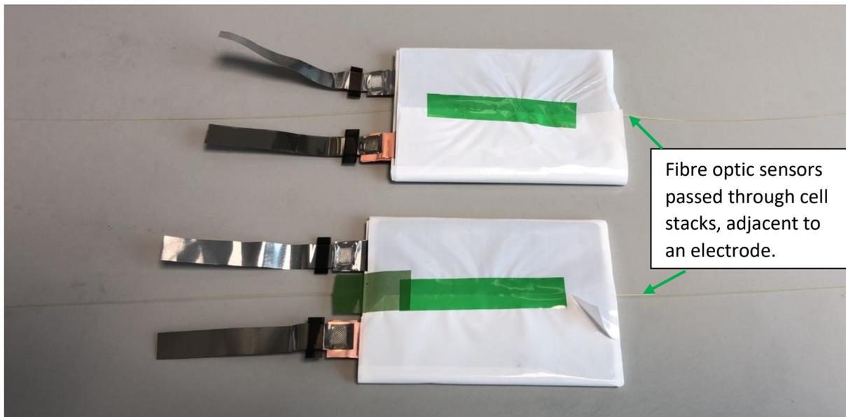
Figure 3-11- Plasmonic based fibre optic sensor fibres introduced through the centre of cell stacks, adjacent to an electrode
