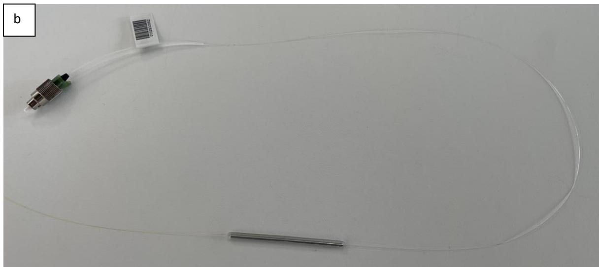
Figure 3-2- a) SPR fibre sensor and pigtail fibre being placed in fusion splicer, b) SPR sensor fibre and pigtail fused with splice protector added
