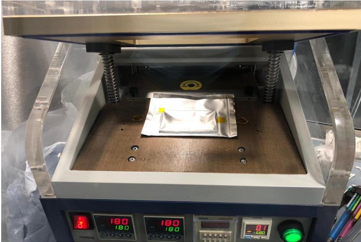
Figure 3-13- A cell with fibre sensor incorporated before final seal under vacuum takes place
