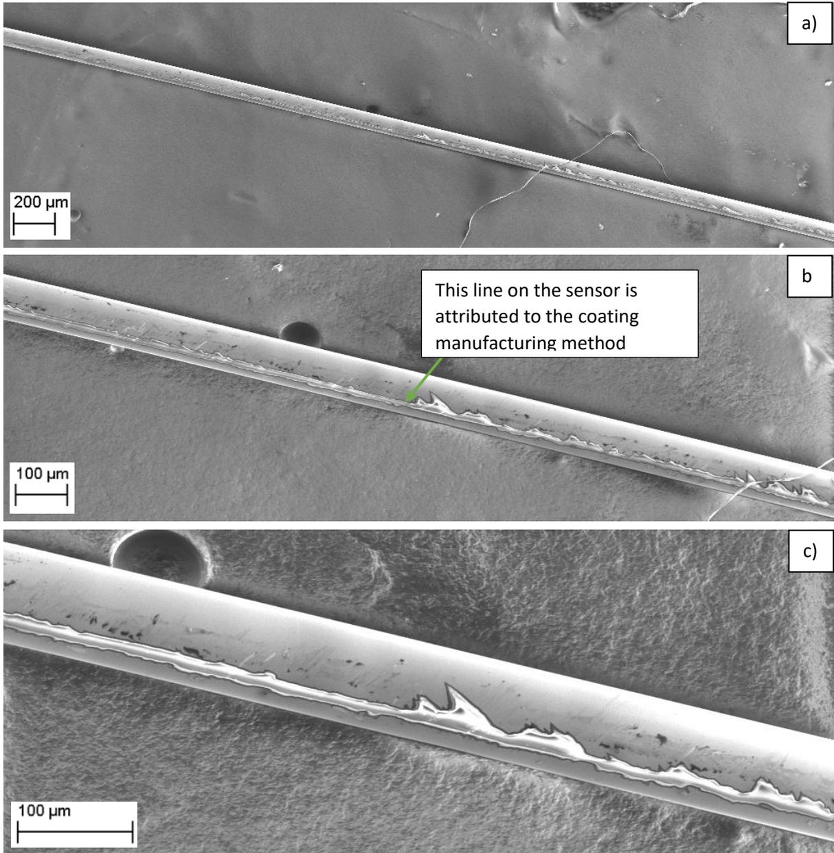
Figure 4-31- SEM images of the sensing region of an unused plasmonic based fibre optic sensor, at magnifications of a) 66x, b) 170x and c) 381x.
