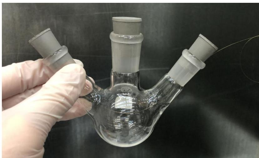
*Figure 3-3- Three neck flask containing a SPR fibre optic sensor*
