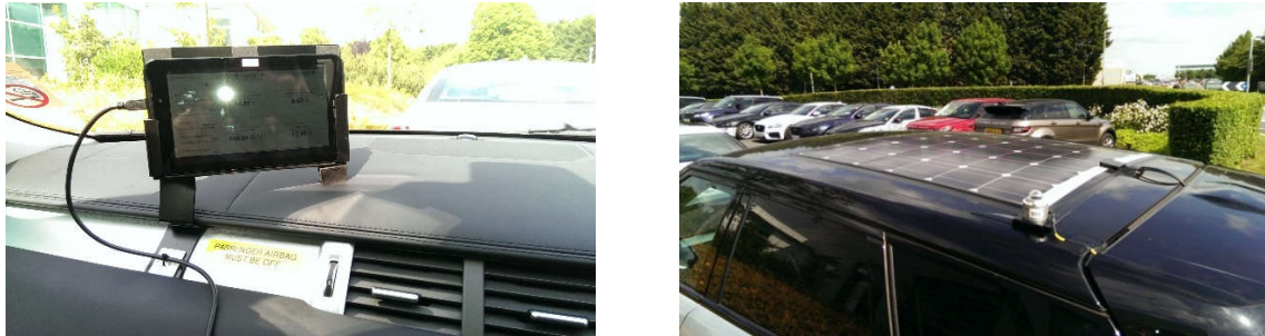
Figure 3.17. ENECOM's Solar Panel as integrated on the LEV's roof
