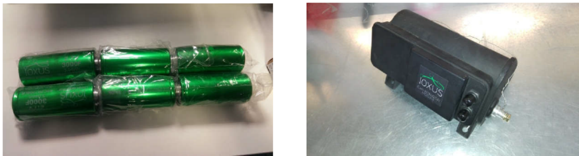
Figure 3.8. IOXUS Single cells of 2.7V and 2700/3000F (left) as included in the 333F module (right)
