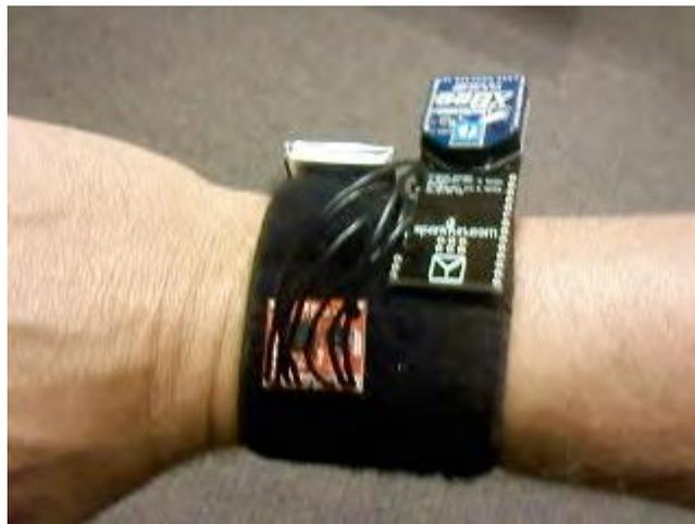
Figure 42 Wearable accelerometer
